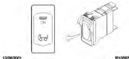
Fig 191, Air-Suspension Dump Valve
