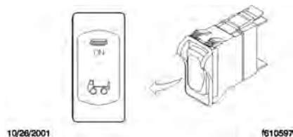
Fig 102, Suspension Dump Switch
