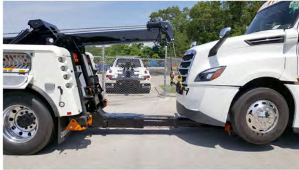
Fig 245, Stinger with Lift Adaptors Under the Axle (tow truck shown)
