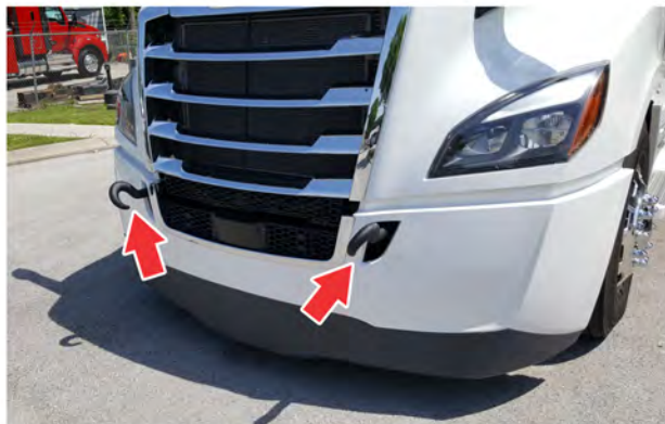
Fig 238, Tow Hooks Installed, Facing Down
